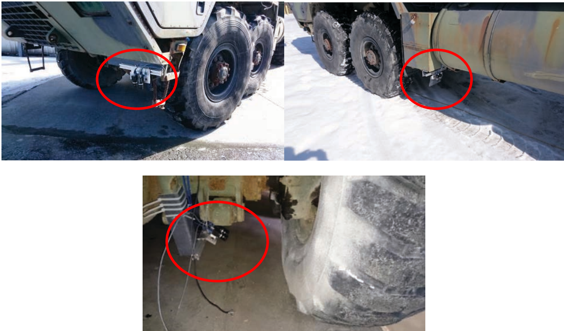
Figure 4: HEMTT camera set mounting locations: front camera set prior to leading tire (top left); rear camera set aft of the second axle (top right); and side camera mounting location in-board of the tire to monitor tire slip (bottom).
